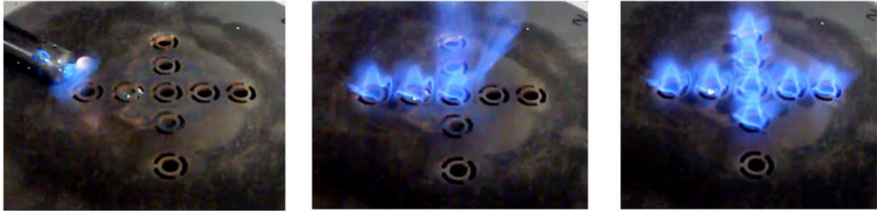
Figure 20: Right Picture Shows Final Port Ignition Failure Due to Large Port Gap Distance
