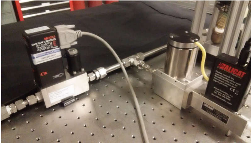
Figure 7: Forced Draft Ring-Stabilizer Air Pre-Mixing Manifold
