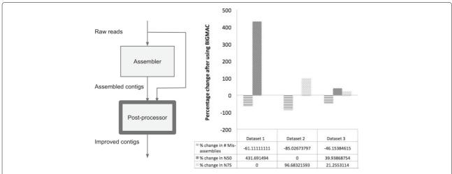
**Fig. 1** Position of post-processor in an assembly pipeline (*left*). Improvement in assembly quality using post-processor BIGMAC on three different datasets (*right*). BIGMAC shows the effectiveness of the post-processing approach for long read metagenomic assembly
