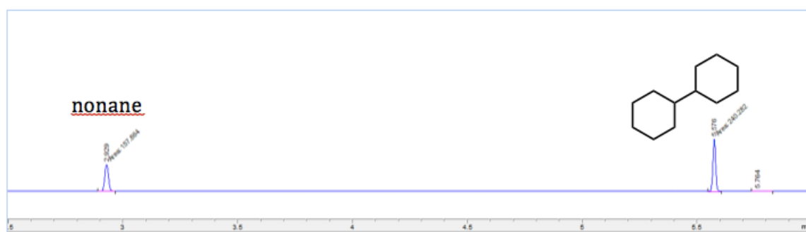
Figure 3.2 GC Trace Showing 1:1 Mixture of Nonane to Bicyclohexyl.
