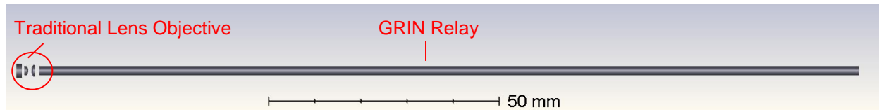
Figure 5-2. Shaded CAD models of two different imaging systems. A. GRIN Objective with GRIN Relay (System 1). B. Traditional Objective with GRIN relay (System 2).
