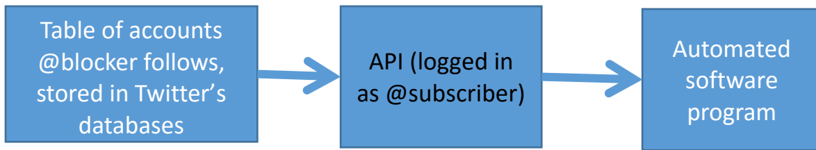
Figure 31: Getting a list of accounts @blocker follows. Information flows from list of accounts on Twitter's databases to the software program
