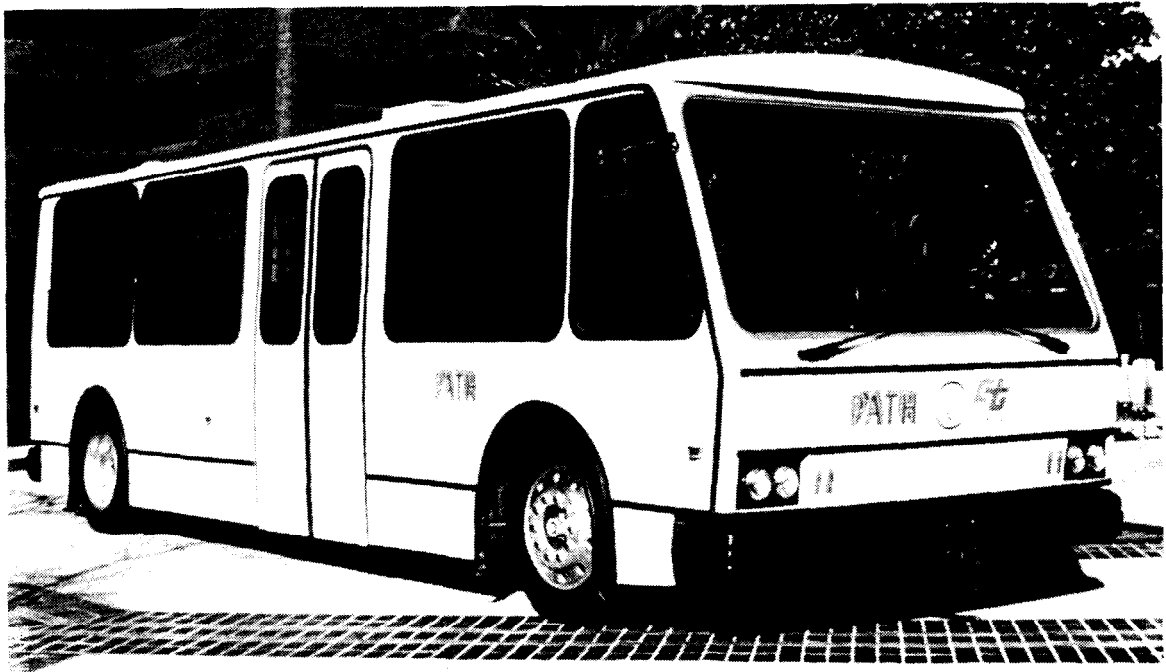
Figure 1.4 Prototype roadway power electric bus
