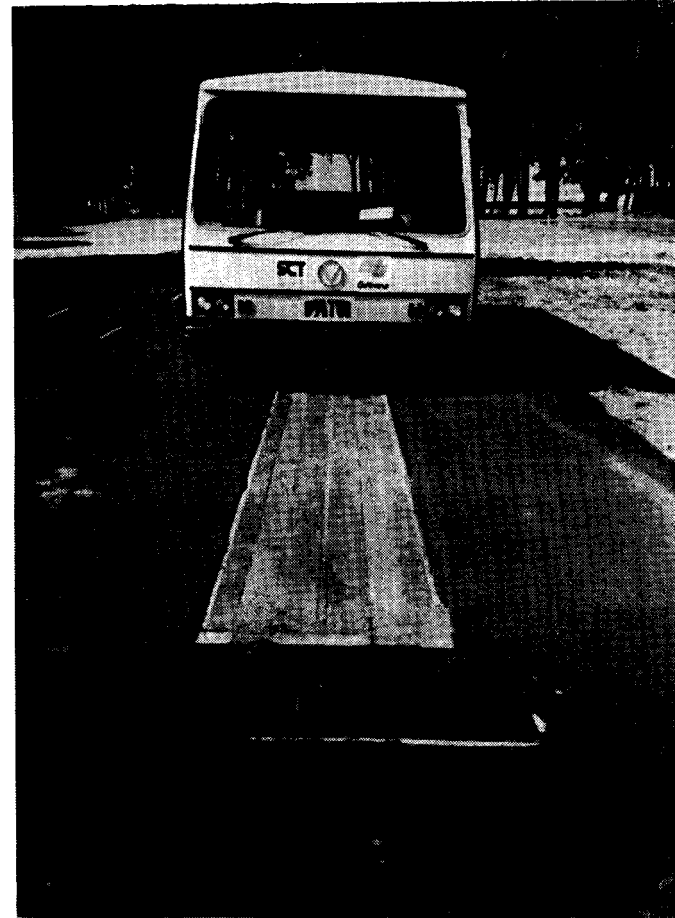
Figure 1.11 Roadway powered electric bus over bus stop
