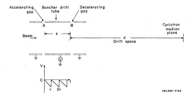
Fig. 1. Proposed drift tube buncher driven by a sawtooth voltage wave, V. Beam is velocity modulated at gaps A and B, to give space bunching at cyclotron median plane after drift distance, d.
