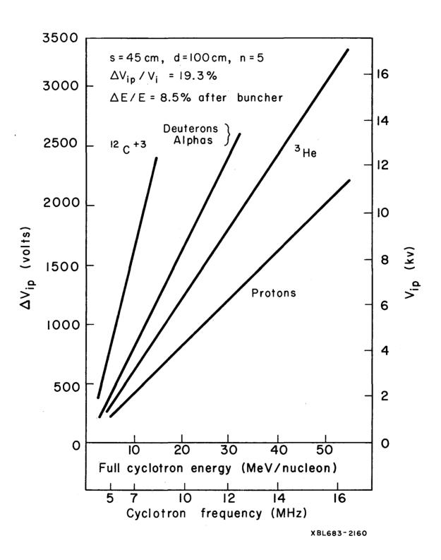
Fig. 4. Buncher voltage  $\Delta V_{ip}$  required for various cyclotron operating energies and particles, using scaled injection energy  $V_{i}$ . Buncher parameters for this typical case are shown.
