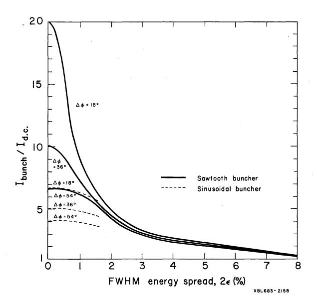
Fig. 6. Ratio of current accelerated by cyclotron for bunched and unbunched cases,  $I_{bunched}/I_{d.c.}$ , for  $\Delta \phi$  full width phase acceptance, for equal d.c. beam from the ion source. Abcissa is the FWHM energy spread  $2\epsilon$ . Comparison is given between sawtooth and sinusoidal wave shapes.
