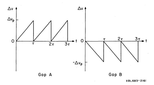
Fig. 2. Velocity modulation,  $\triangle v$ , given to particle at gap crossings A and B. Gap B partially cancels out the effect of gap A.
