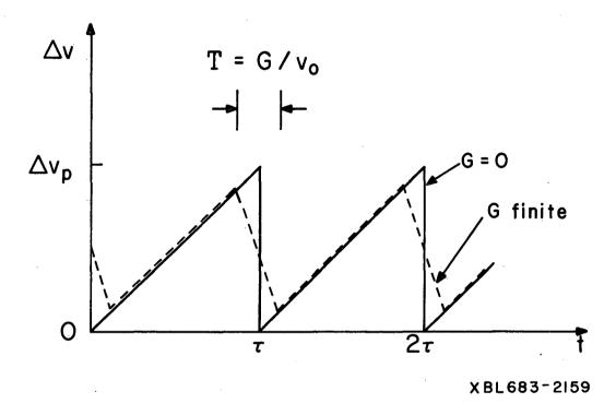
Fig. 5. Comparison of velocity modulation,  $\Delta v_{\text{\tiny J}}$  at buncher gap for cases of zero gap width and gap width G.
