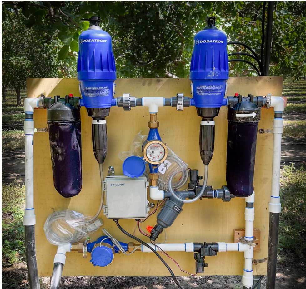
Figure 6: Fertigation system designed to operate without grid power in the center of an irrigation run and be operated remotely. Two valves are actuated via a SIM-enabled controller that also broadcasts data from the two flow sensors. Each dosatron injector handles a treatment and feeds the corresponding lines to the treatment layout.
