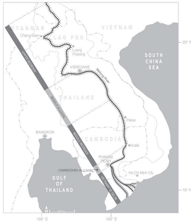
Figure 3. Reaches of predominantly bedrock vs alluvial channel from Rubin et al. (2014). Bedrock-controlled channel reaches are likely to experience rapid loss of surficial sediment deposits, but will not manifest large channel changes in response to reduced sediment loads, whereas alluvial reaches will likely incise and/or widen as they erode to compensate for reduced sediment supply.
