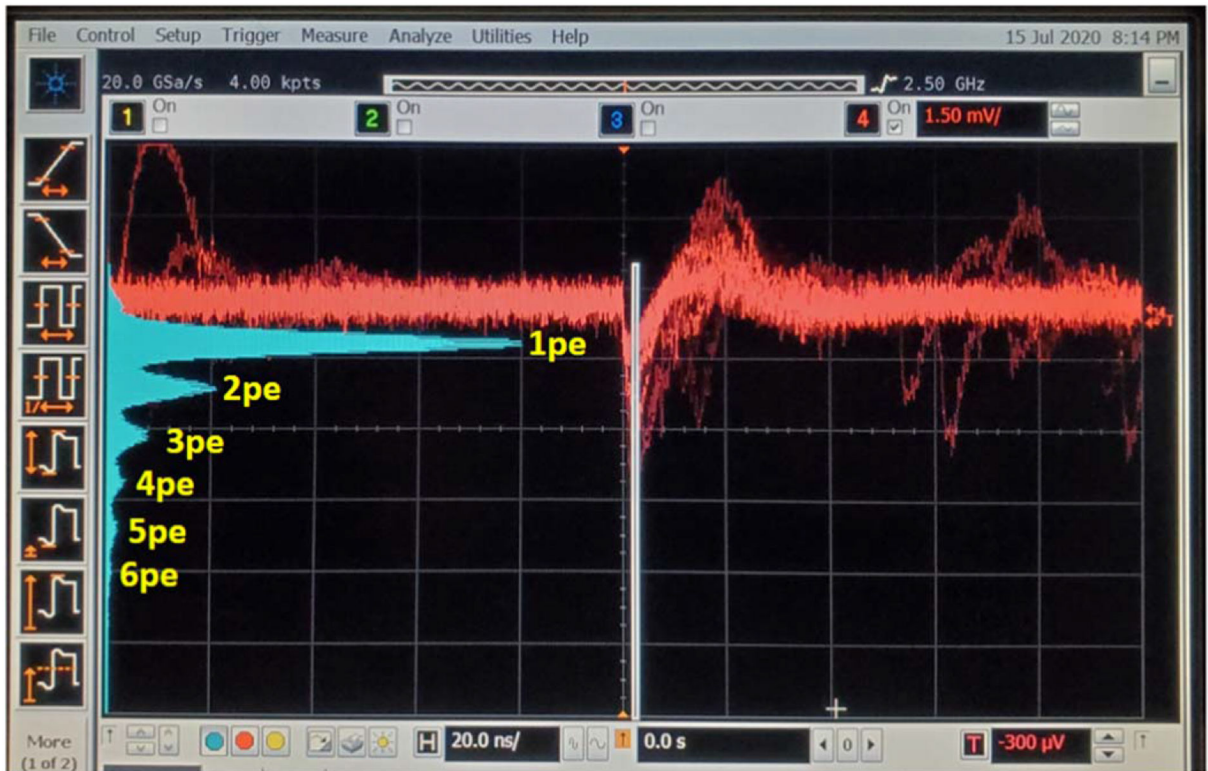
Figure 5. Single photon charge spectrum (SPCS, shown in blue) of amplified timing signal for our prototype TOF-PET detector. The amplified timing signal is shown in red; the x -axis is the time (ns) and y -axis is its amplitude (mV).
