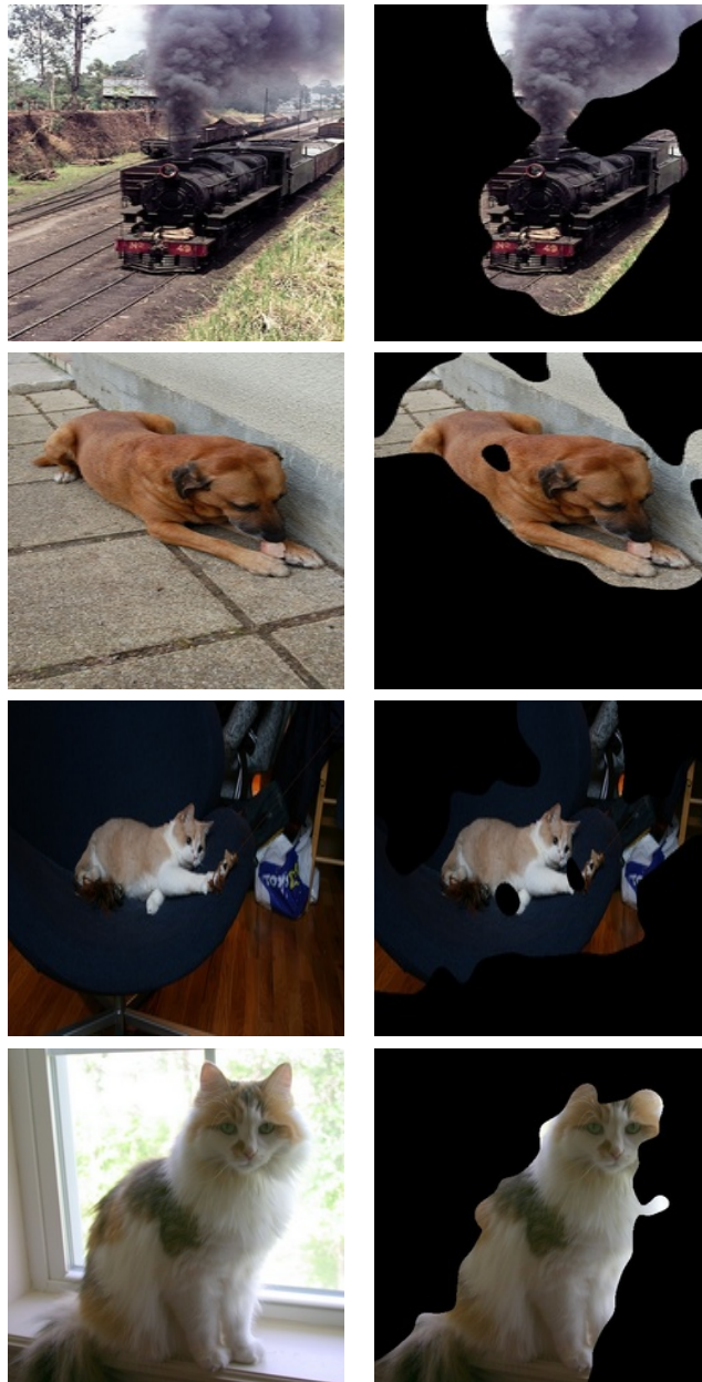
Figure 3.4: Some examples of selective attention image masking based on Ventral Net sensitivity analyses. The first column shows original images, and the second column displays the results of Ventral Net based masking.
