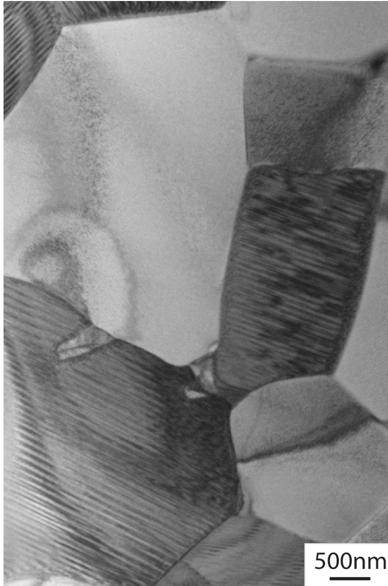
Figure 7.6 BF-TEM image indicates that after 100h at 1500°C, twinned M -YT (dark contrast) and t -ZrO 2 (light contrast) are present in 28Y28Ta.
