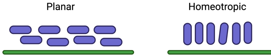
Figure 2.7: Schematic view of planar and homeotropic anchoring. In planar anchoring, liquid crystals' molecules are parallel to the boundary, and in homeotropic, they are perpendicular to the substrate.
