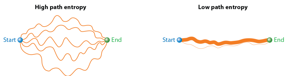
Figure 2. Path entropy measures the uniformity of the traffic distribution through different routes. Line thickness indicates the traffic density, i.e., pathway probability.
