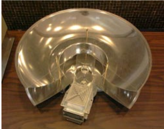
Figure 3. Cut away photograph of bi-phase, non-contiguous reflector.
