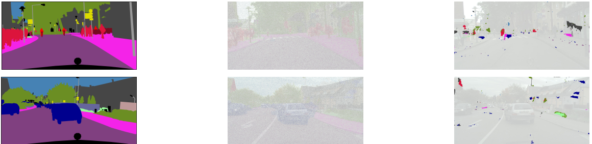
Figure 2.2: Qualitative visualization of pixels annotated by the human oracle for GTAV \rightarrow CITYSCAPES. From left to right. Ground truth maps, pixels annotated by random selection, and pixels annotated by uncertainty based selection.
