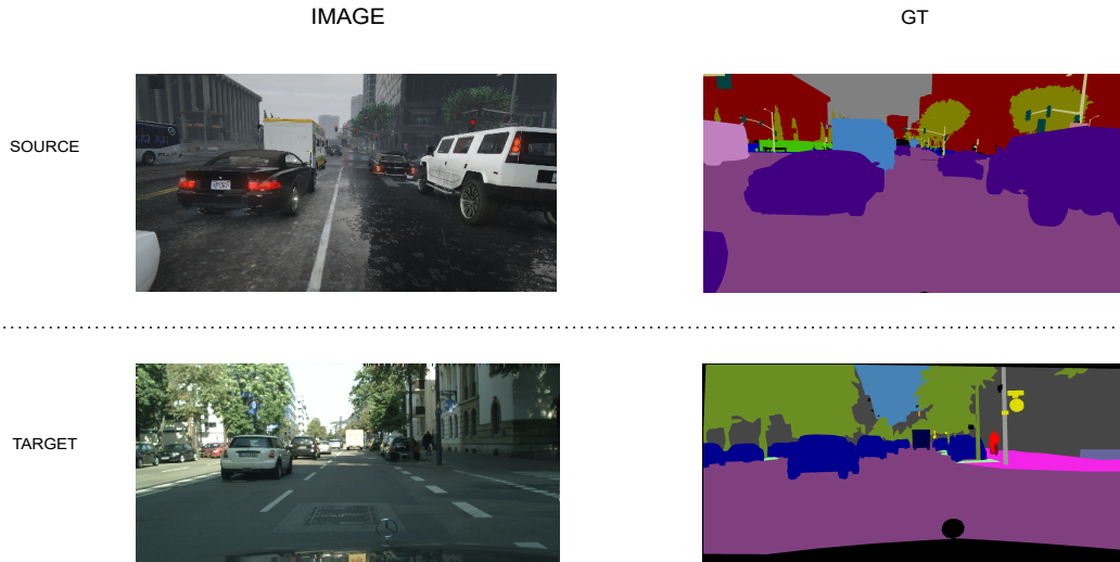
Figure 1.1: Figure depicting the visual domain gap between the GTAV(Source) [45] and Cityscapes(Target) dataset [13]. GTAV is a dataset of synthetic images and Cityscapes reflect real-world imagery. A model trained on synthetic images will fail to capture the semantic concept in real-world urban imagery.
