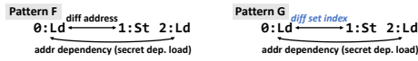
Figure 13: (F) Pattern using default grammar (Tab. 4). (G) More precise pattern after adding the diffindex predicate.
