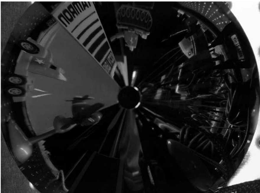
Fig. 8 Best-focus picture, Casio QV2000UX, f=6.5\text{mm} , F/8 , 1/2 sec, indoor office ceiling fluorescent light.
