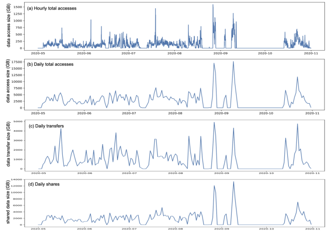
Figure 15: Network traffic size on ESnet node; (a) hourly total data access size, (b) daily total data access size, (c) daily data transfer size, (d) daily shared data size
