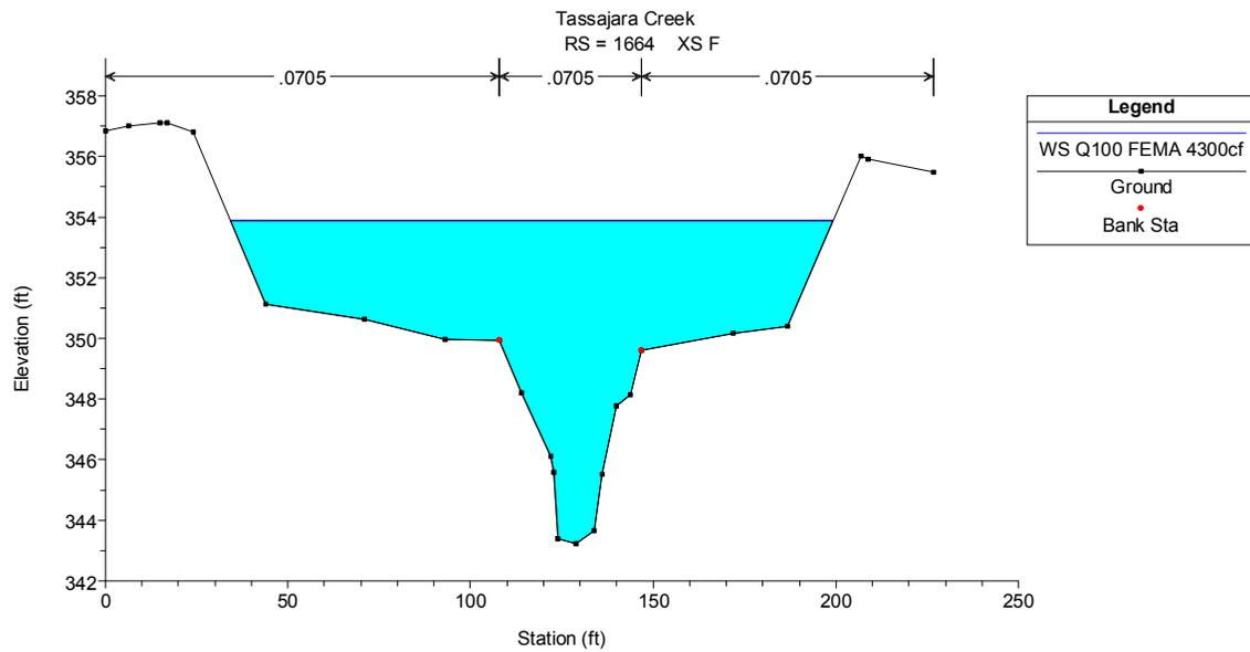
**Figure 32. Cross-Section G at 4,300 cfs (FEMA Q<sub>100</sub>)**
