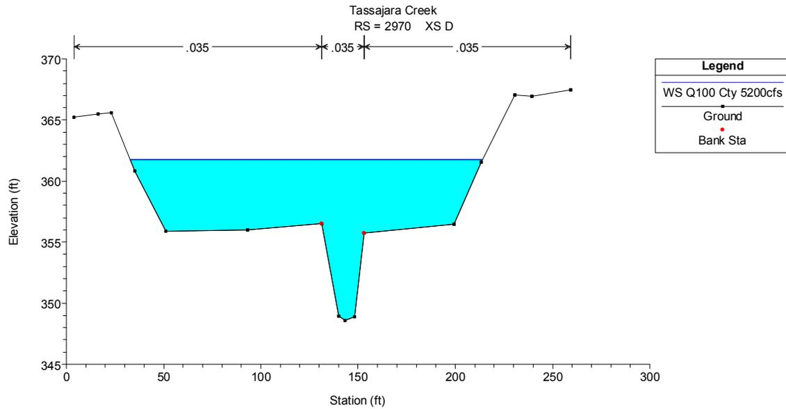
**Figure 37. Cross-Section E at 5,200 cfs (AC Q<sub>100</sub>)**
