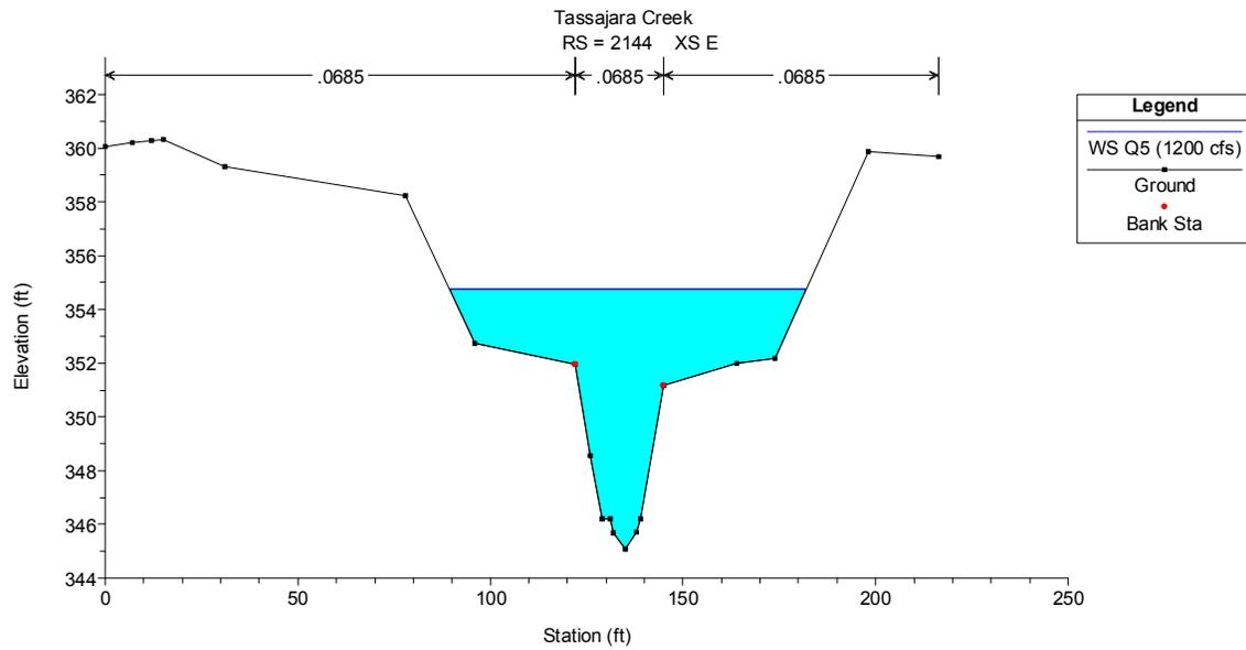
**Figure 18. Cross-Section F at 1,200 cfs ( $Q_5$ )**
