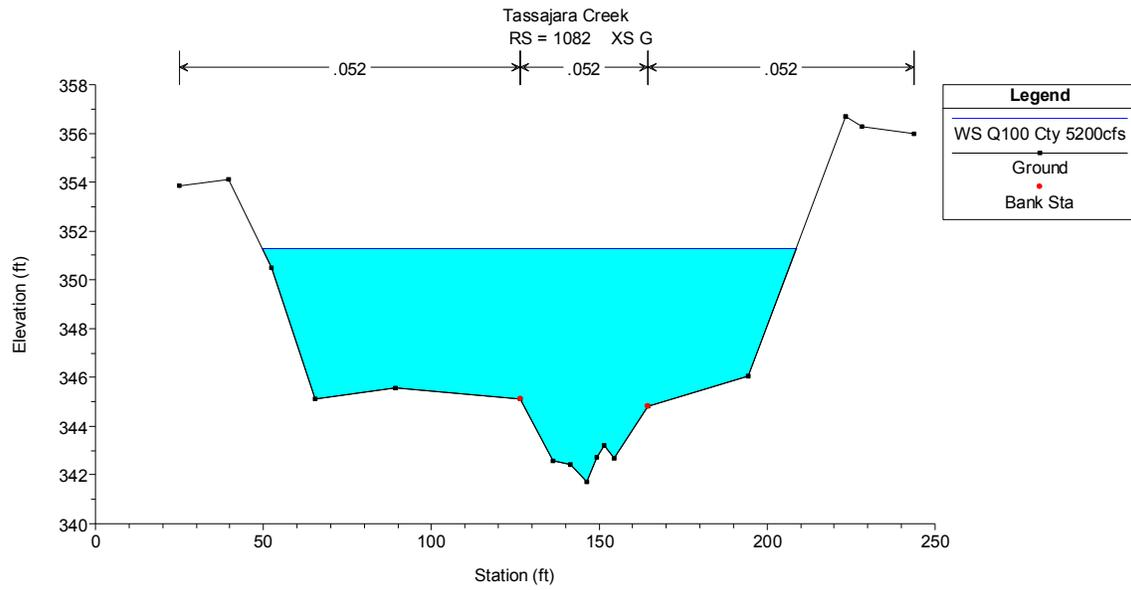
Figure 40. Cross-Section H at 5,200 cfs (AC Q<sub>100</sub>)
