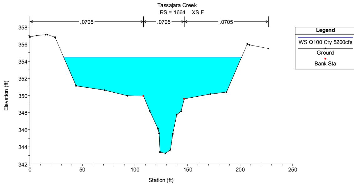
Figure 39. Cross-Section G at 5,200 cfs (AC Q<sub>100</sub>)
