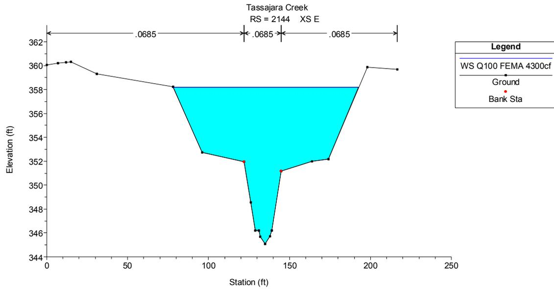
Figure 31. Cross-Section F at 4,300 cfs (FEMA Q<sub>100</sub>)
