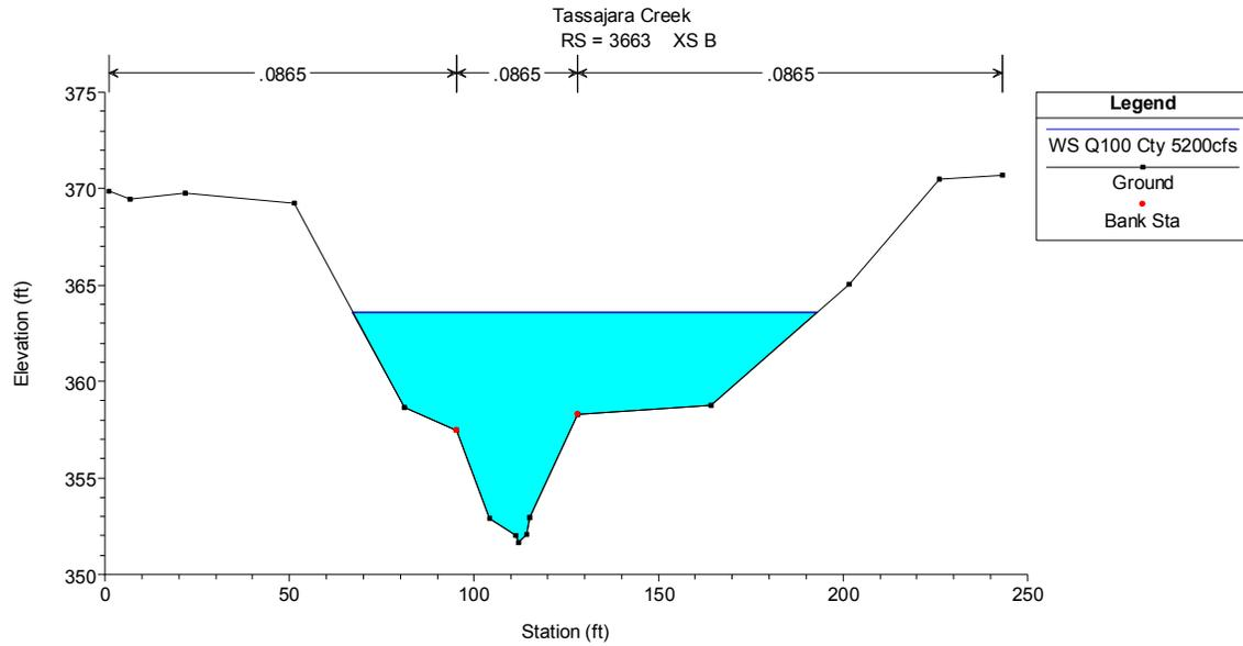
**Figure 36. Cross-Section D at 5,200 cfs (AC Q<sub>100</sub>)**
