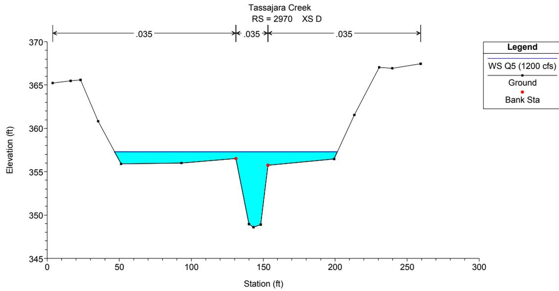
Figure 17. Cross-Section E at 1,200 cfs ( $Q_5$ )
