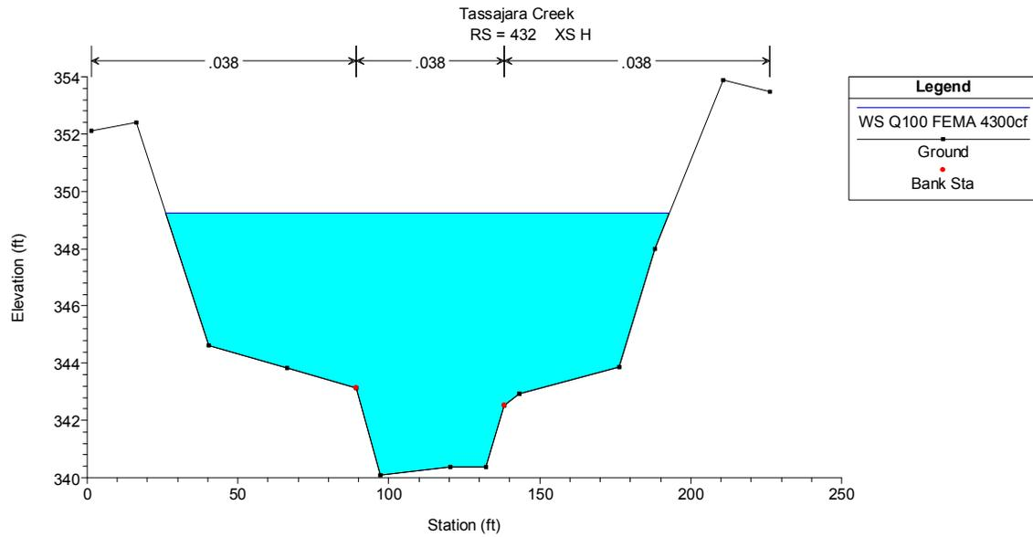
**Figure 34. I-580 at 4,300 cfs (FEMA Q<sub>100</sub>)**
