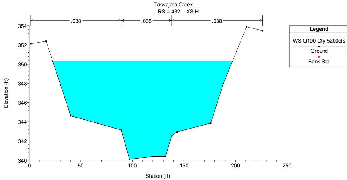
**Figure 41. I-580 at 5,200 cfs (AC Q<sub>100</sub>)**
