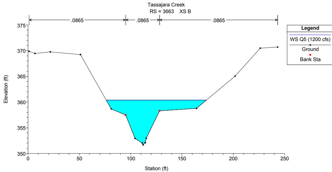
Figure 16. Cross-Section D at 1,200 cfs ( $Q_5$ )
