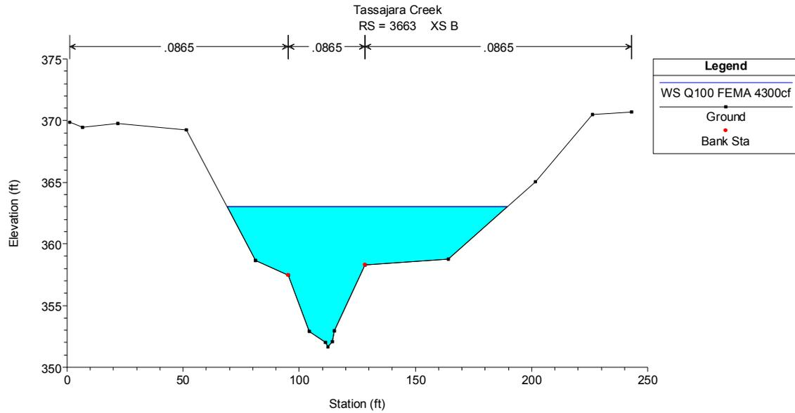
**Figure 29. Cross-Section D at 4,300 cfs (FEMA Q<sub>100</sub>)**
