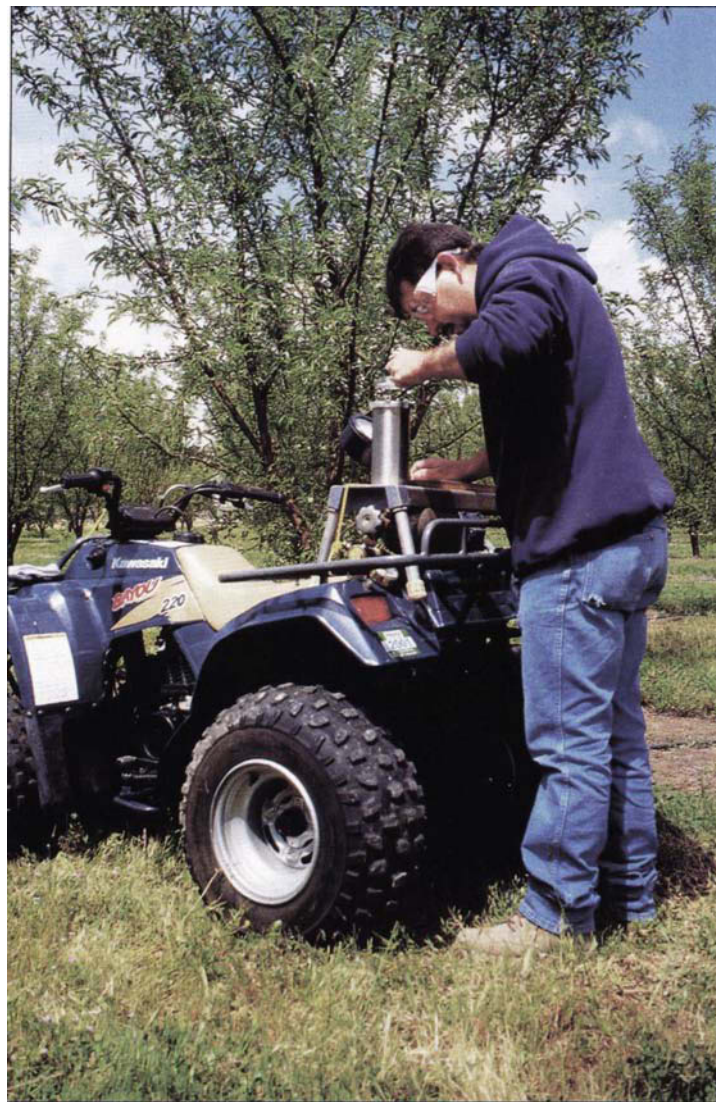
Mario Salinas takes pressure chamber measurements with the console model used in this study. This relatively large type of pressure chamber can be mounted on an all-terrain cycle for easy orchard access.
