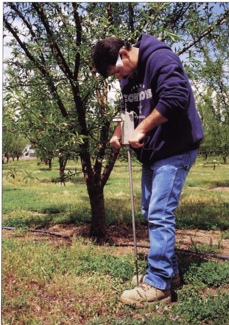
An alternative to the console model pressure chamber is this “pump-up” type (PMS Instrument Co., Corvallis, OR) where pressure is generated manually, much like using a tire pump.
