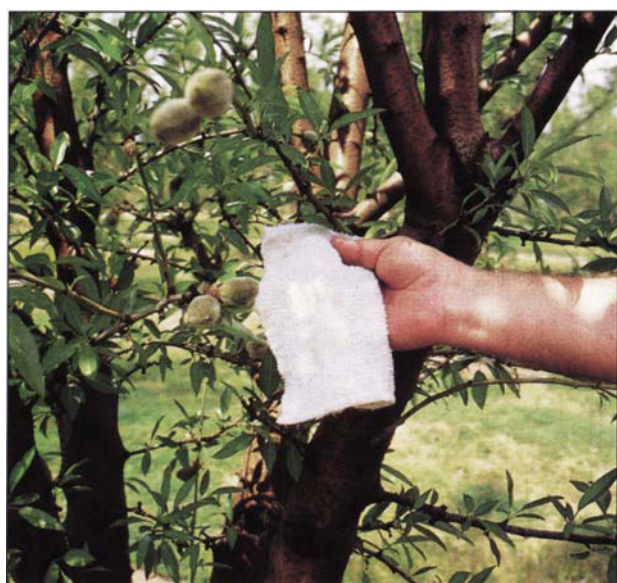
One advantage of the technique for measuring shaded leaf water potential (LWP) outlined in this paper is that shaded leaves need only be covered by a damp cloth for the short time between excision and placement of the leaves in the pressure chamber.
