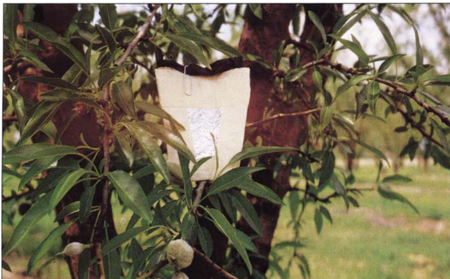
Leaves close to the trunk must be covered by small, foil-covered plastic bags for a period of time prior to measuring stem water potential (SWP).
