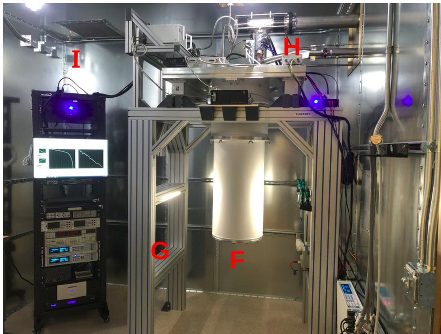
Figure 7.6: Photos of the LBNL refrigerator. Top is open, back view; bottom is closed, front view. **A**: 4K Flange, **B**: Still Flange, **C**: Cold Plate Flange, **D**: Mixing Chamber Flange, **E**: Mixing Chamber, **F**: Closed Fridge, **G**: Anti-Vibration Mount, **H**: Room-Temp Inputs, **I**: Filtered Power Banks.
