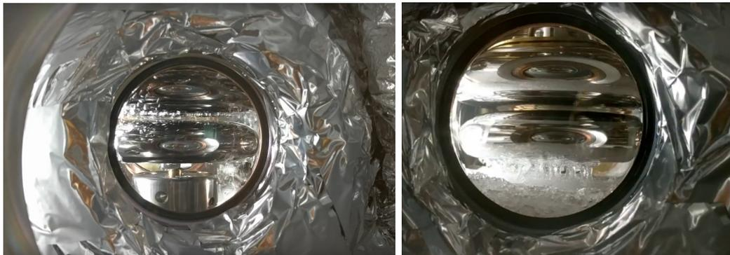
Figure 3.3: Photographs of xenon, taken with the Xenon Breakdown Apparatus experiment (XeBrA) [87]. (*Left*) Bubbling in liquid xenon. (*Right*) Solid xenon accumulated at the bottom of the chamber. Note that in a properly functioning dark matter detector, neither bubbles nor solid xenon should be present in the liquid xenon chamber. Images screenshotted from videos taken by Lucie Tvrznikova [88, 89].
