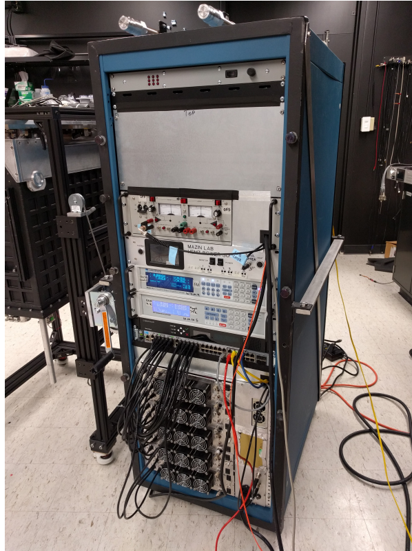
Figure 3.14: DARKNESS electronics rack in lab at UCSB. This rack holds 5 readout cartridges with 10 sets of the readout boards described in Section 3.4, 2 per cartridge, installed in a custom readout crate at the bottom of the rack that distributes power, 1 PPS, and 10 MHz signals to the boards. Above the crate is a network switch, time source, thermometry control, HEMT power supply, and ADR magnet power supply.
