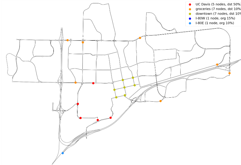
Figure 5. Traffic demand in the morning. Popular areas are weighted for sampling OD nodes.
