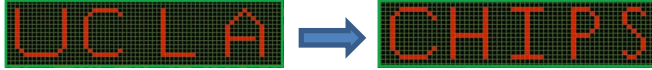
Fig. 5. Bitmaps of a fully functional CTT memory array integrated in 14nm FinFET technology: A ‘UCLA’ pattern was written followed by an erase and re-write of a ‘CHIPS’ pattern.
