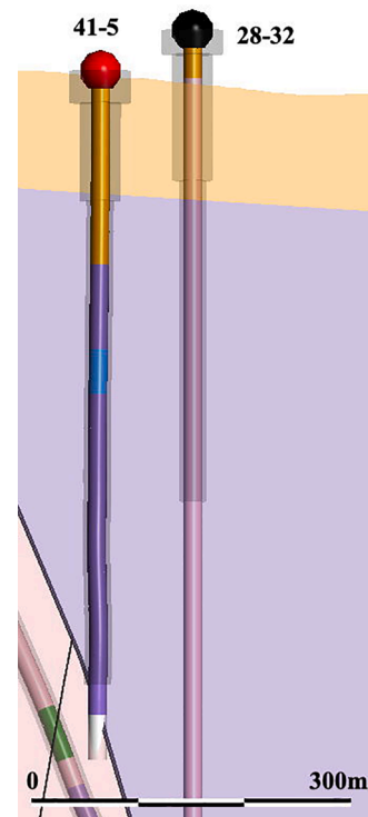
Fig. 13. 3D geologic model schematic of Well 41-5. Stratigraphy and blind drilling indicating LC. Orange is Tertiary volcanics, green is Paleozoic metasediments, purple is predominantly clay minerals, and white is blind drilling. Note that the LC zone is associated with the intersection of the well with the fault zone (dark gray). Cased intervals are shaded gray.
