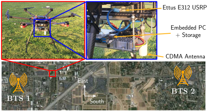
Fig. 13. SOP BTS environment and experimental hardware setup for the UAV experiment. Map data: Google Earth.
