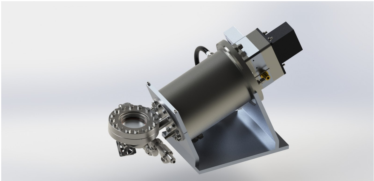
Figure 6.11: New generation API neutron generator built and tested by Adelphi Inc. [1]. Several improvements were made to allow for a superior position resolution and the ability to handle higher alpha rates among others.
