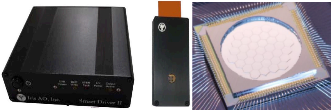
Figure 2. [Left]: Presentation of the PTT111 and its driver [Right]: Surface view of the PTT111 DM (Iris AO).
