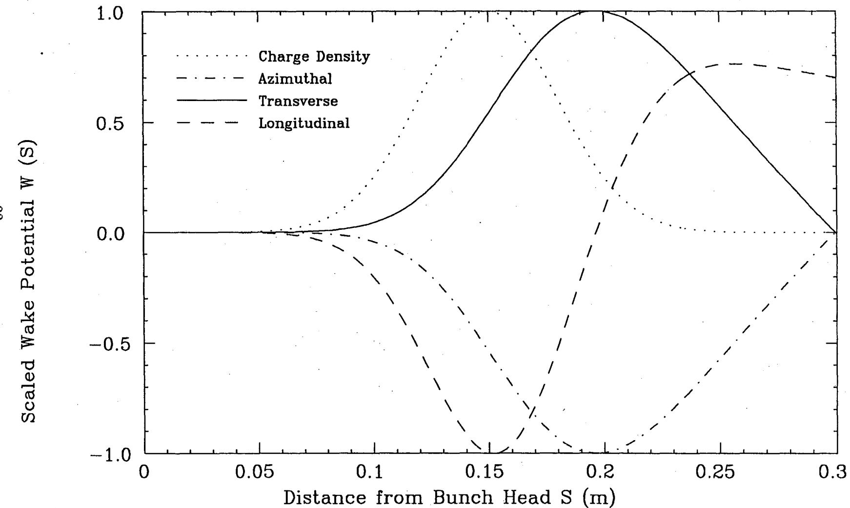
Azimuthal Wake Min/Max= -5.779E+00/ 3.559E-01 V/pC/m, Loss Factor= -3.092E+00 V/pC/m
