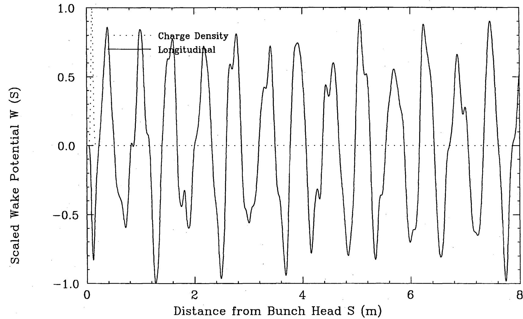
Longitudinal Wake Min/Max= -4.786E-01/ 4.362E-01 V/pC, Loss Factor= -2.821E-01 V/pC
