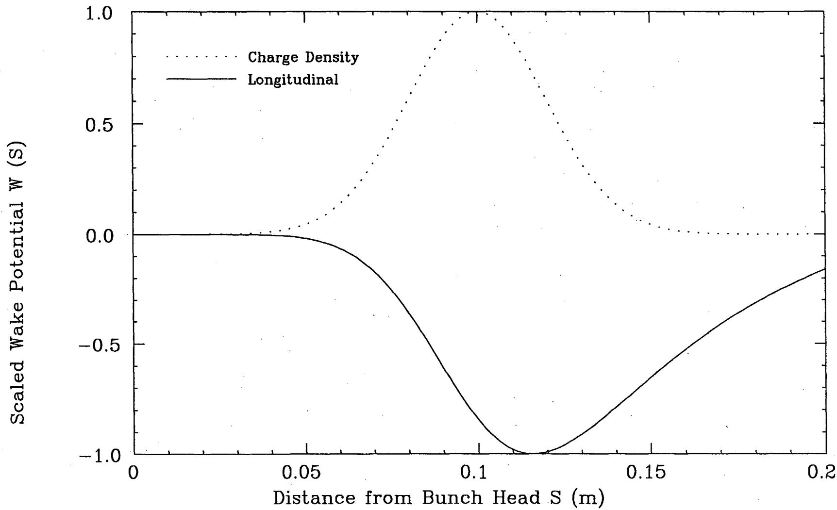
Longitudinal Wake Min/Max= -3.910E-01/ 0.000E+00 V/pC, Loss Factor= -2.785E-01 V/pC
