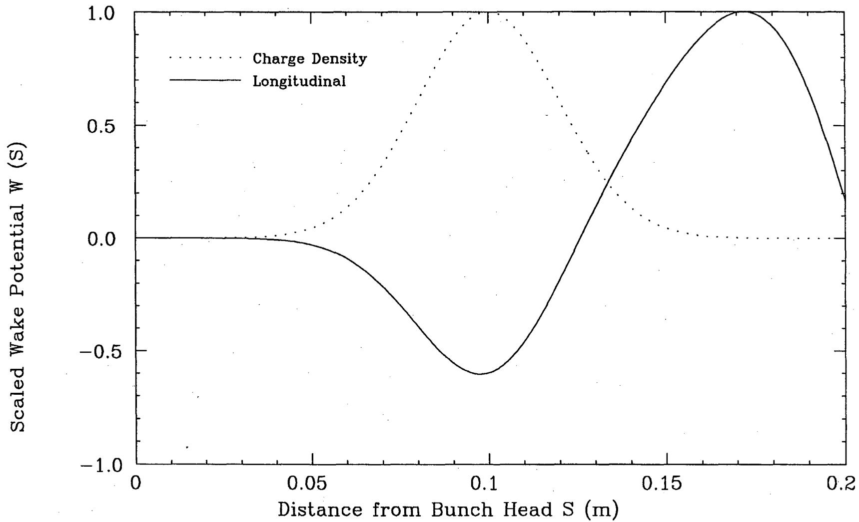
Longitudinal Wake Min/Max= -7.094E-01/ 1.176E+00 V/pC, Loss Factor= -4.180E-01 V/pC
