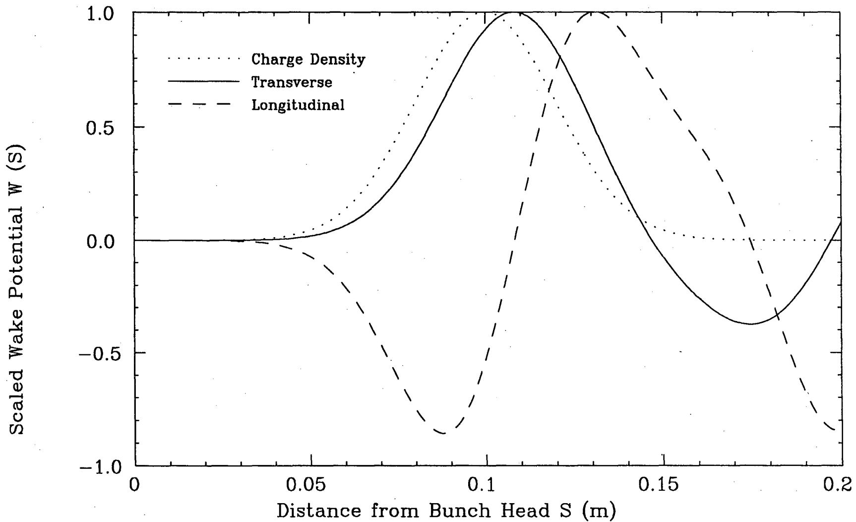
Transverse Wake Min/Max= -3.747E+01/ 9.950E+01 V/pC/m, Loss Factor= 6.736E+01 V/pC/m
