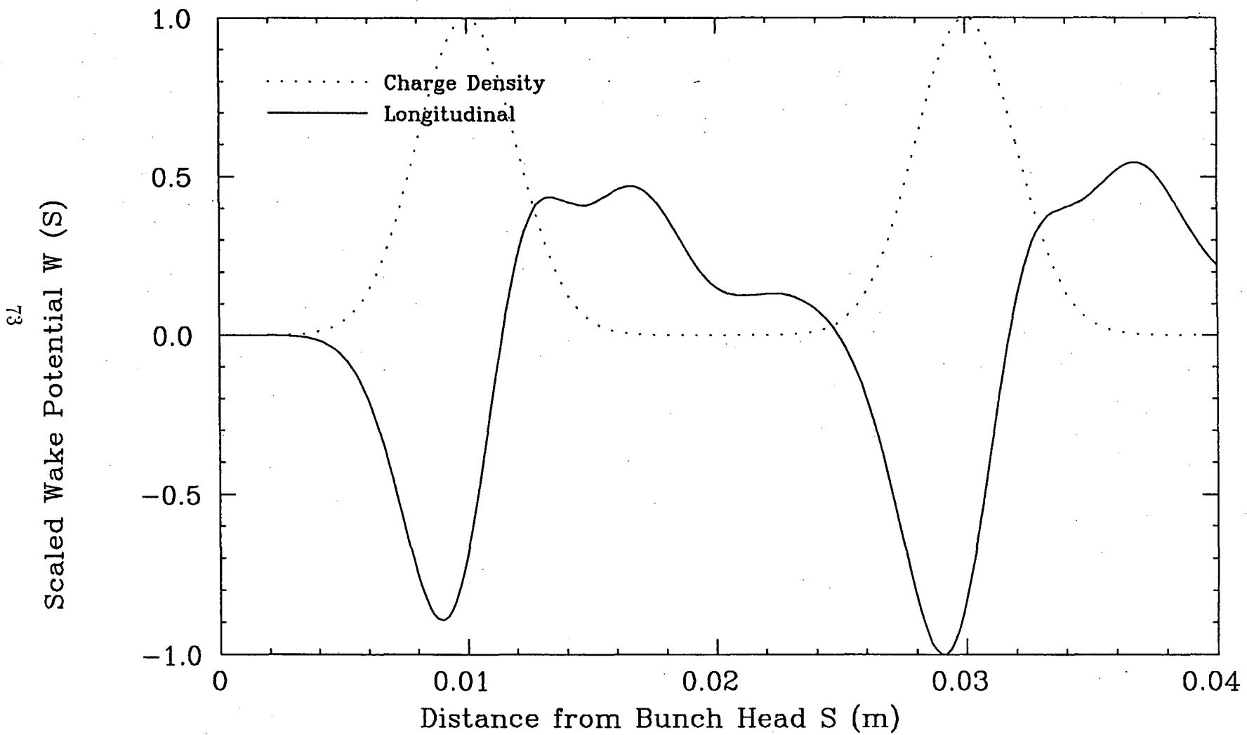
Longitudinal Wake Min/Max= -2.395E-01/ 1.298E-01 V/pC, Loss Factor= -1.045E-01 V/pC
