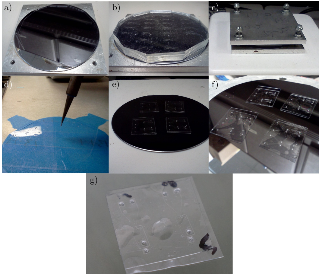
Figure 3.13: Images of Device fabrication and bonding. a) Plastic film on silicon wafer ready for embossing. b) PDMS stamp in place. c) Stamp and plastic film in fixture on hot plate. d) Completed embossing and adding fluidic pass-throughs with a soldering pencil e) Devices on another plastic film for bonding. Four sets of two devices. f) Post-bonding of devices. g) Image of two bonded devices.
