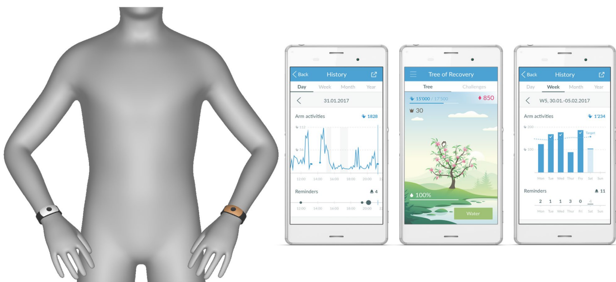
Fig. 1 The motion-tracking devices and phone application used for the measurements. The application was designed to allow the tracking of arm activity counts over the day, week, and month. Silver tracker: “ARYS™ me|tracker” for the paretic wrist; Golden tracker: “ARYS™ pro|tracker” for the non-paretic wrist
