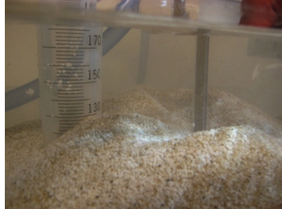
Fig. 5 A picture of the Scour Net being tested in a wet environment is shown. The experiment entailed placing a sensor in close proximity of the model graduated cylinder bridge pier
