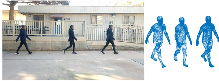
Figure 2.2: (Right) Three sample HMR algorithm output meshes for (left) different snapshots of a walking person.
