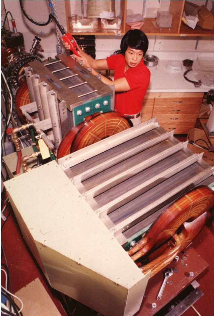
Figure 4: Wobbler magnets – 1-meter long dipoles with sinusoidally-driven fields that produce circular beam patterns at patient site, 5 meters downstream (towards lower-right). Field sizes of \pm 2\% uniformity, up to 30 cm diameter could be obtained by overlapping several circles of different radii.
