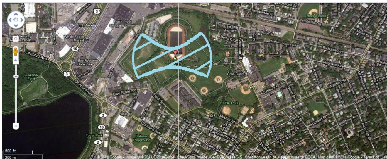
Figure 13: Expected topography of shadow flicker effect (indicated by blue stripes) over Danehy Park at one particular wind turbine site for the Northern Power 100.
