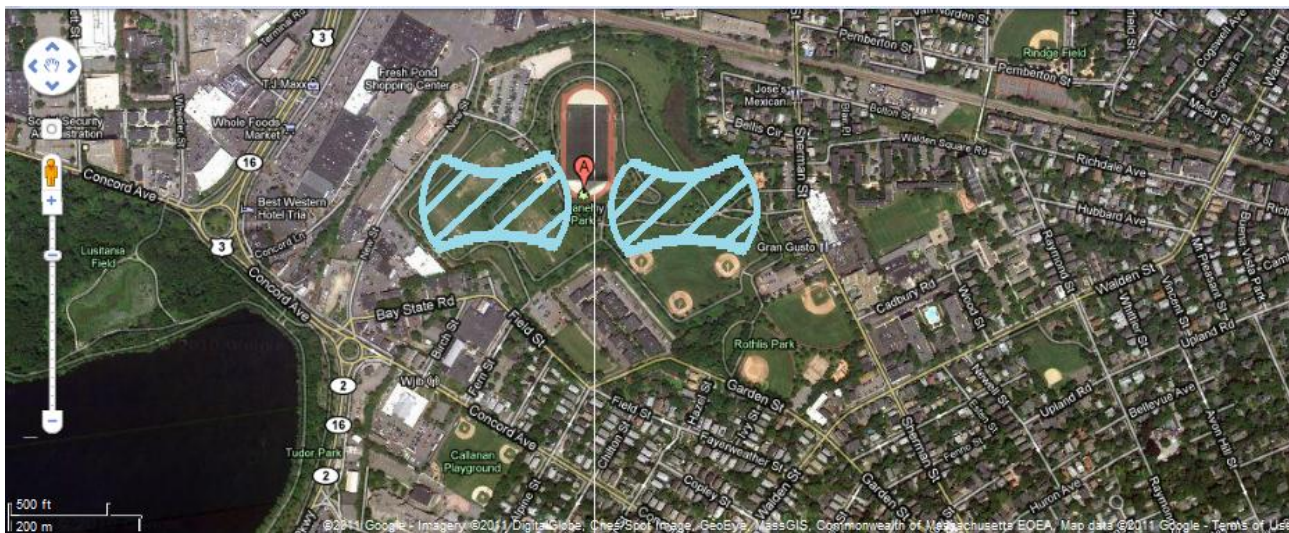
Figure 11: Expected topography of shadow flicker effect (indicated by blue stripes) over Danehy Park at various particular wind turbine sites for the Polaris P10-20.
