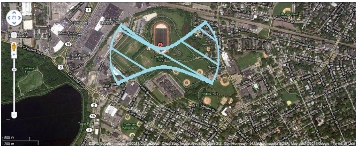
Figure 1: Expected topography of shadow flicker effect (indicated by blue stripes) over Danehy Park at one particular wind turbine site for the Aeronautica 29-225.
