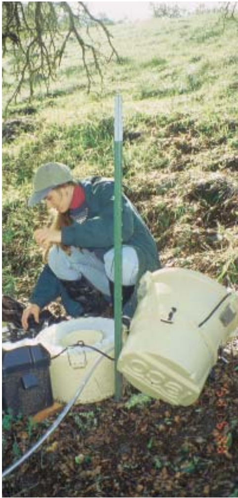
Preliminary data indicate that current land use and management practices are not impairing water quality on the seven experimental watersheds. Julie Smith monitors automatic water samplers.
