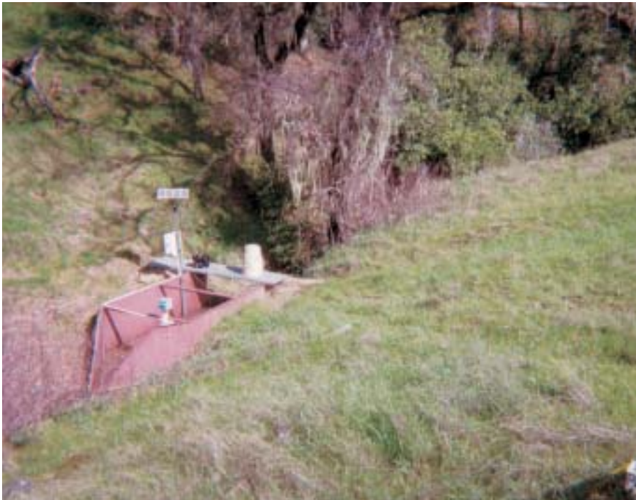
Stream flow and water-quality sampling equipment are located at the outlet of each experimental watershed. In coming years, studies will focus on the roles that grazing and fire management play in plant communities, hydrology and water quality.
