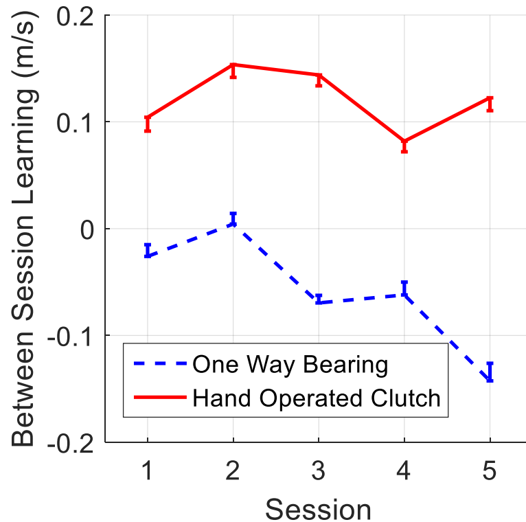
FIGURE 2.5B: BETWEEN-SESSION VELOCITY CHANGE OF EACH GROUP. THE HAND CLUTCH GROUP SHOWED BETWEEN-DAY LEARNING, WHEREAS THE ONE-WAY BEARING GROUP DID NOT. ERROR BARS SHOW \pm 1 STANDARD ERROR.
