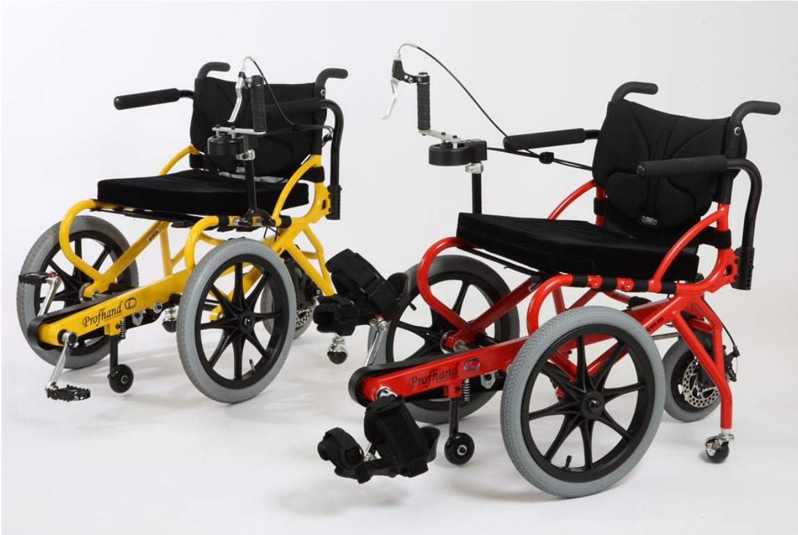
FIGURE 1.4: A COMMERCIAL PEDAL WHEELCHAIR FOR LEG EXERCISE IN STROKE PATIENTS [96].
