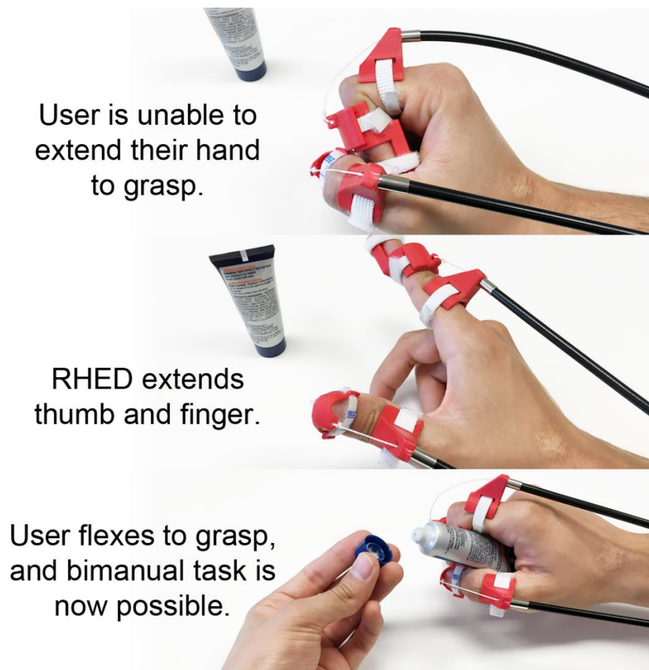
FIGURE 5.3: EXAMPLE USES OF RHED IN ACTIVITIES OF DAILY LIVING. HERE THE USER ALLOWS RHED TO ASSIST IN OPENING A TUBE, SOMETHING A PERSON WITH STROKE WOULD HAVE GREAT DIFFICULTY DOING.
