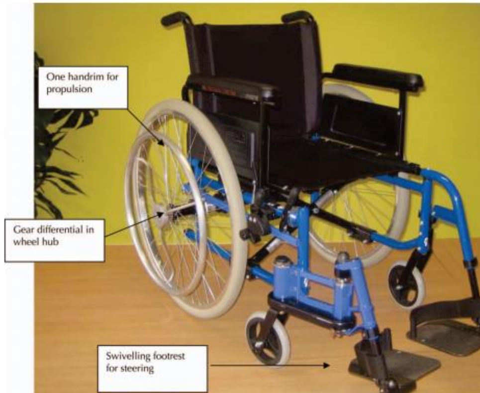
FIGURE 1.3: A MODIFIED WHEELCHAIR DRIVEN BY ONE HAND AND ONE FOOT FOR STROKE PATIENTS, TAKEN AS IS FROM [82].
