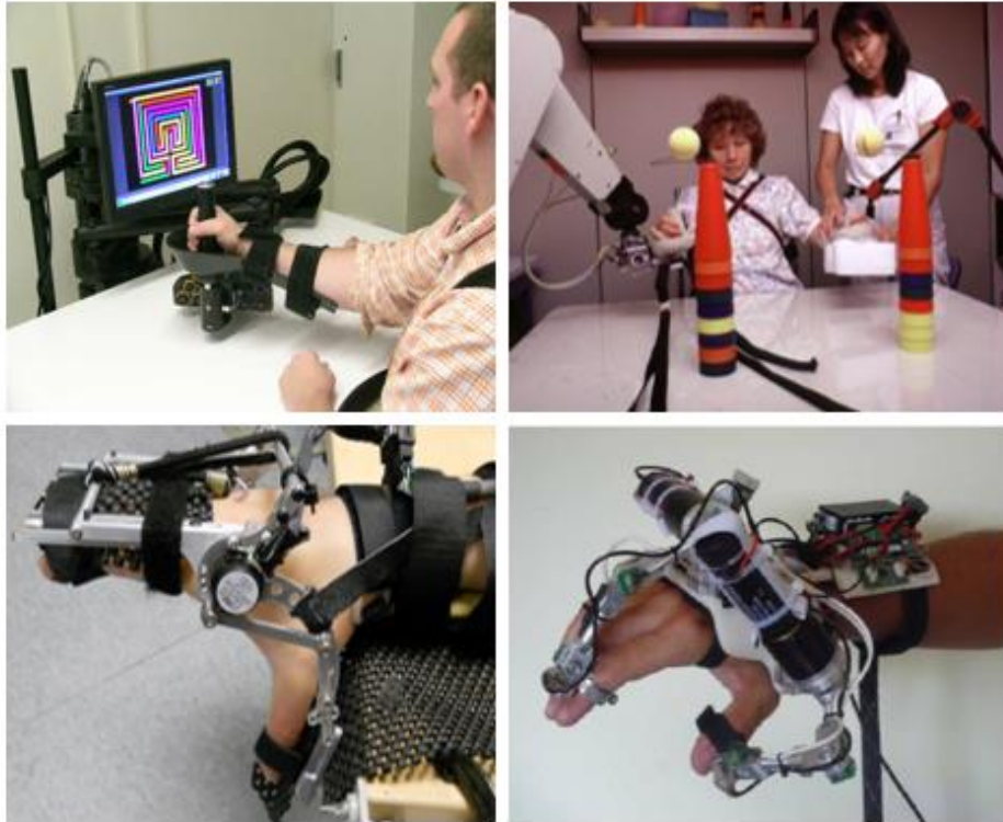
FIGURE 1.1: EXAMPLES OF UPPER EXTREMITY ROBOTIC TECHNOLOGIES. TOP LEFT: THE MIT-MANUS. TOP RIGHT: THE MIME ROBOT. BOTTOM LEFT: HANDSOME, A PASSIVE HAND EXOSKELETON. BOTTOM RIGHT: HEXOSYS, AN ACTIVE HAND EXOSKELETON.
