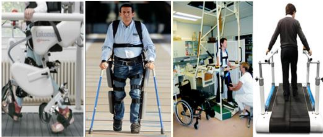
FIGURE 1.2: LOWER EXTREMITY ROBOTIC TECHNOLOGIES. FAR RIGHT: THE LOKOMAT, A STATIONARY NATURAL GAIT ROBOTIC DEVICE. MIDDLE RIGHT: THE REWALK OVERGROUND NATURAL GAIT ROBOTIC DEVICE. MIDDLE LEFT: THE GAIT TRAINER, A STATIONARY ALTERNATE GAIT ROBOTIC DEVICE. FAR LEFT: A SPLIT-BELT TREADMILL, A STATIONARY ALTERNATE GAIT ROBOTIC DEVICE.
