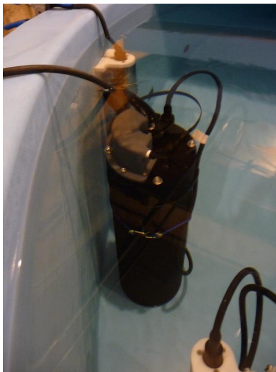
Figure 2.30. Preliminary test tank deployment with autonomous sensor package.
