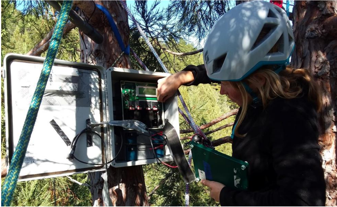
Figure 5: Monthly maintenance of monitoring equipment included retrieving SD cards and changing batteries.
