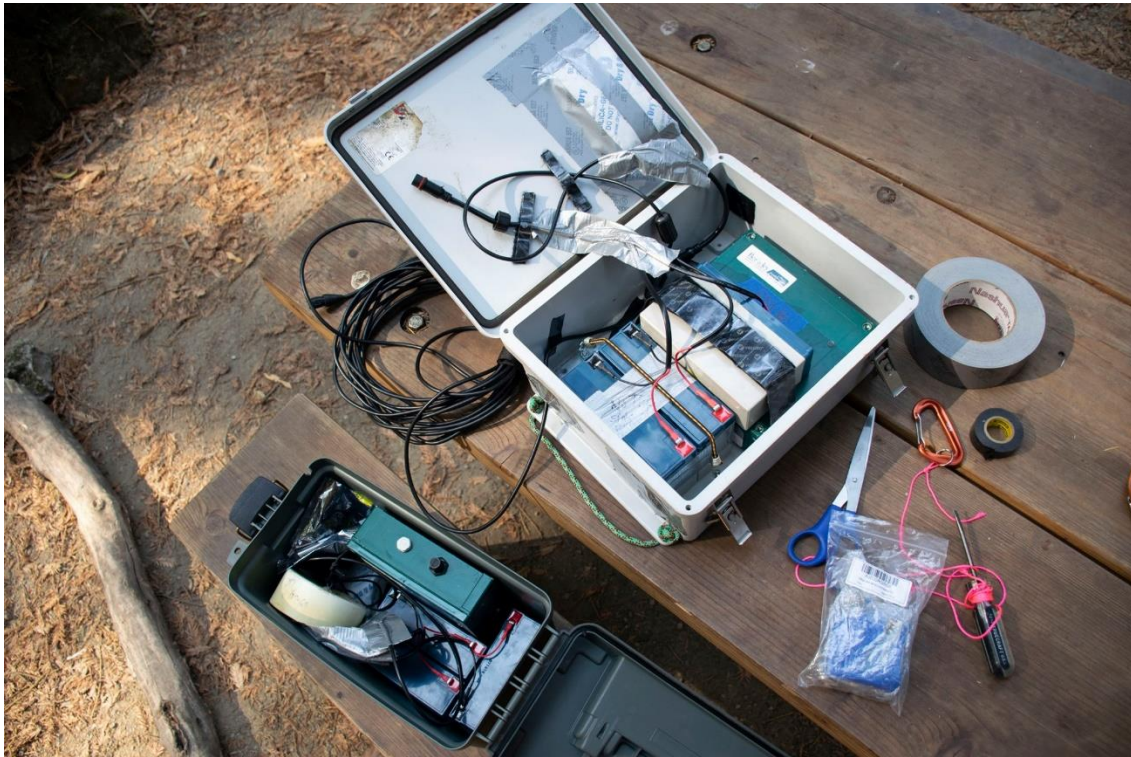
Figure 6: SM2 detectors in weatherproof cases for ground and treetop.
