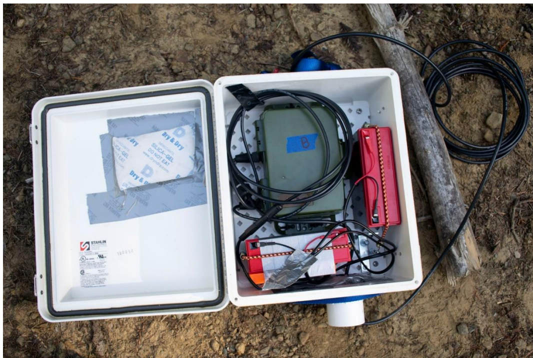
Figure 8: SM4 detector set up for treetop detectors.
