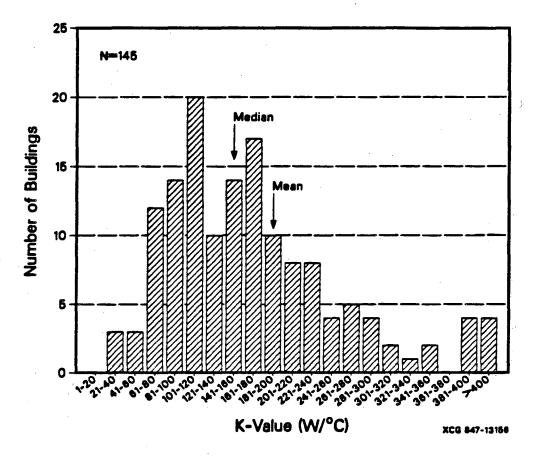
Figure 2. Distribution of k-values for 145 low-energy houses with  $R^2 > 0.50$  and t.  $\leq 20^{\circ}C$ . The mean value was 188 Watts/ $^{\circ}C$ , while the median value was 156 watts/ $^{\circ}C$ . Note that a k-value derived from measured energy consumption data and average monthly temperatures includes the contribution of infiltration, and to a limited extent solar gain and thermal storage.
