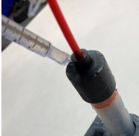
Figure 23: Silicone injection into the dilator cap
