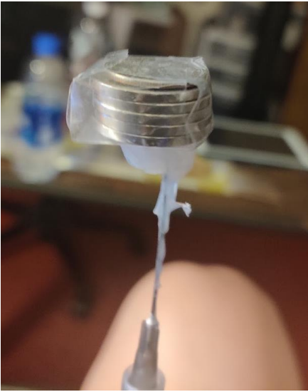
Figure 18: Test for Return Force of the Actuator
