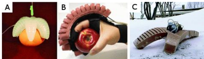
Figure 1: Example of Soft Robotics. A) A soft gripper actuated by pneumatics. [1] B) A glove that helps the user grip objects by adding additional force to the movement to the user. [2] C) A quadruped robot that is able to move by actuating specific parts [3]
