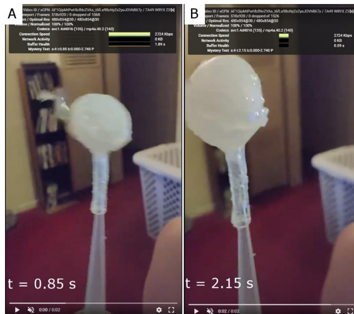
Figure 14: Measurement of the Speed of the Actuator. A) Full contraction occurs at 0.85 seconds B) Return to the original state occurs at 2.15 seconds.
