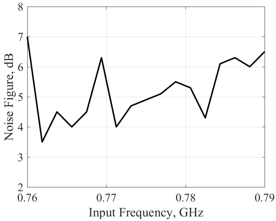
Figure 3.2-4. Measured noise figure of the open loop correlator with varactor biased at -2.8V , reference/carrier power of 28dBm at 4.3GHz .
