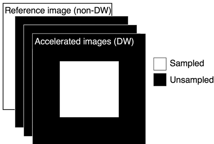
FIGURE 1 Masks for retrospective undersampling of k-space. In Experiment 1, masks in 2D were generated based on random sampling with a Gaussian distribution along the first and second phase-encoding directions (in-plane). The central region and the readout dimension (through-plane) were fully sampled. The number of remaining k-samples was equal to the total number of samples in 3D divided by the acceleration factor, A_{dw} . In Experiment 2, the masks retained only the central region of k-space, where the number of samples in each dimension were down-sampled by a factor of A_{dw}
