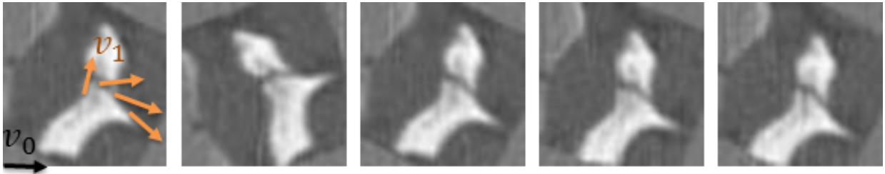
Figure 4. Illustration of 2D patches aligned along the candidate edge orientation with respect to the origin for training convolutional networks (ConvNets).
