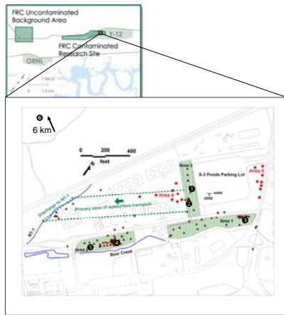
Figure 2. Map of the FRC background area and contaminated site. Inset area shows location of sampled wells. Numbers correspond to Table 1.
