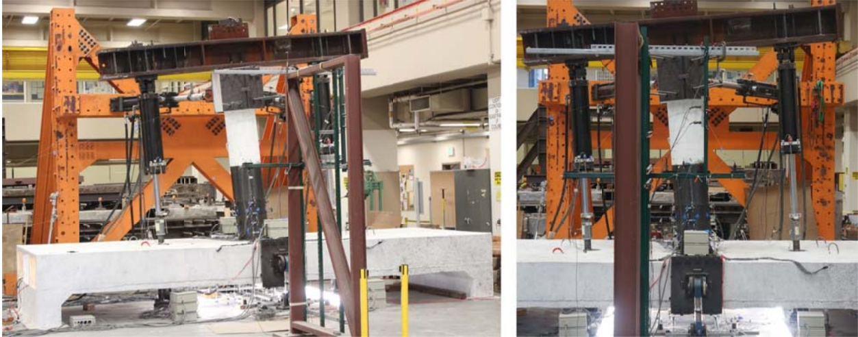
Figure 6.13 Overview of repaired SP1 cyclic loading test setup when loading is in progress and applied in longitudinal direction
