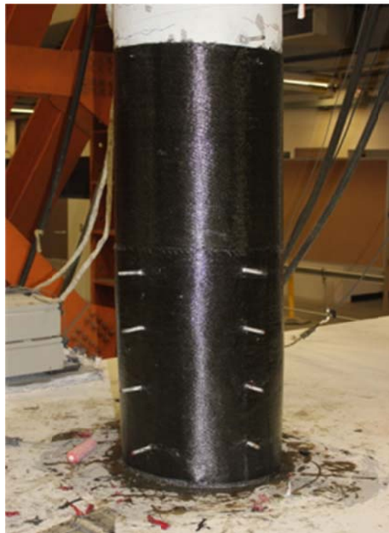
Figure 6.11 Final repaired column after it was wrapped by three CFRP layers
