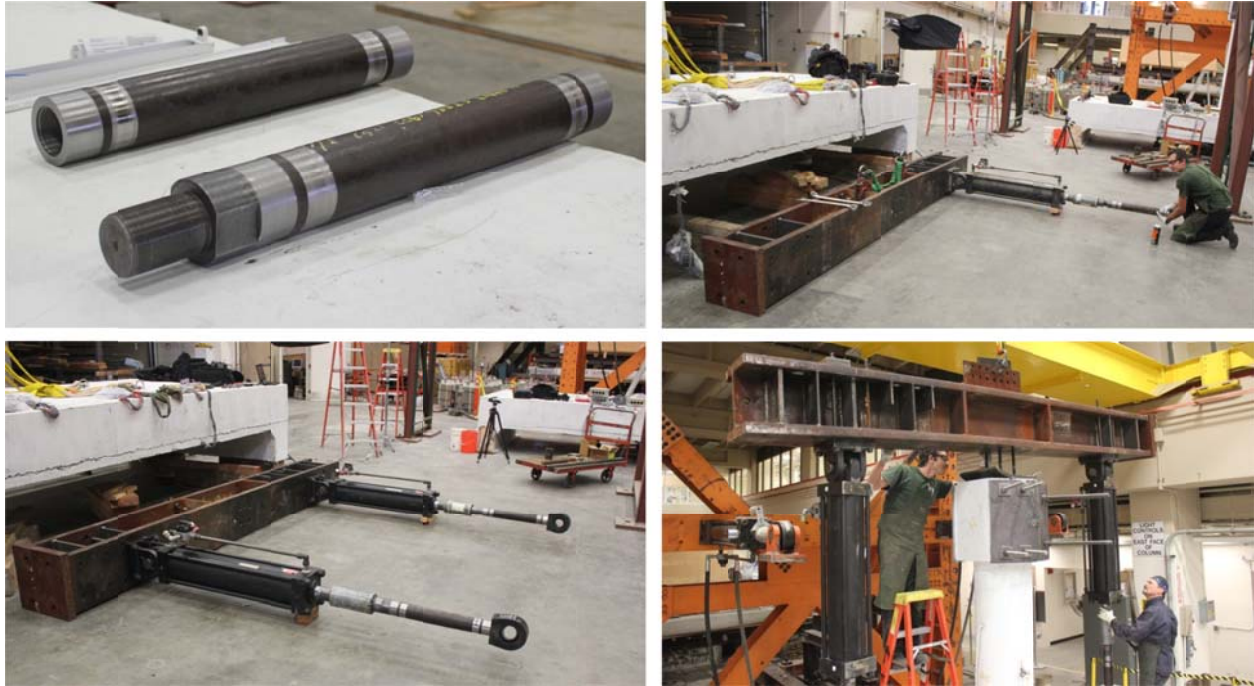
Figure D.9 Different stages of assembling the vertical gravity loading system by assembling the actuators extensions (top left) then attaching the actuators to the spreader beam (top right and bottom left); then moving the whole gravity loading system by the overhead crane to install it on top of the column (bottom right)
