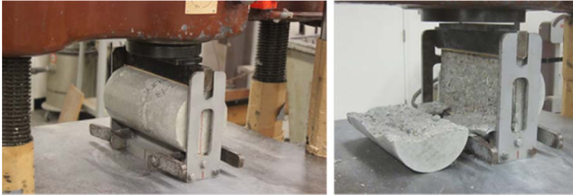
Figure 3.29 Splitting tension test setup (left) and typical mode of failure (right)
