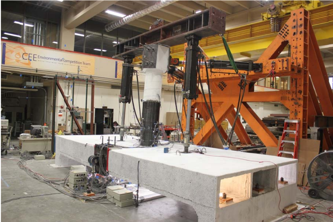
Figure 8.6 Retrofitted SP2 HS test setup during a bidirectional run
