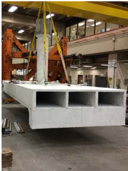
Figure D.4 Moving the first specimen from where it was constructed to where it was tested using the laboratory overhead 10-ton crane
