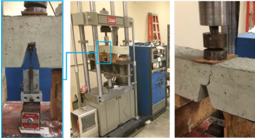
Figure 3.32 Notched-beam test setup, instrumentation, and mode of failure
