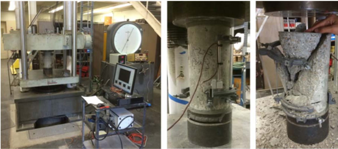
Figure 3.27 Compressive test under displacement control at the University of California, Davis (left), compressometer (middle) and typical mode of failure (right)
