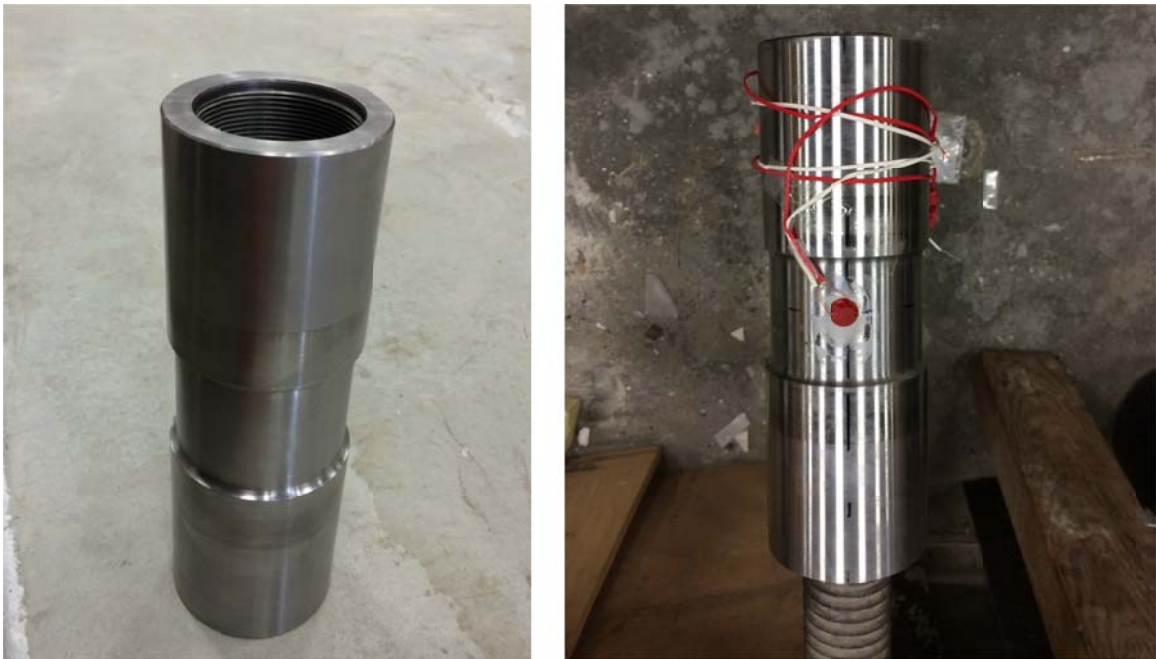
Figure E.3 Final fabricated vertical strut (left) and installing a rosette strain gage (right)
