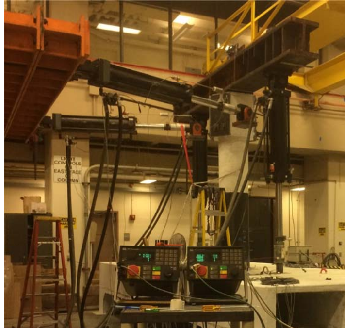
Figure 7.14 Actuators detached from the specimen for conducting trial HS tests
