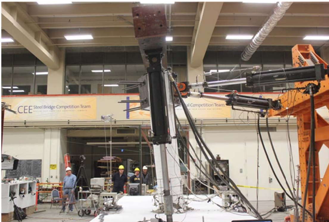
Figure 3.15 A view of first specimen test in progress under transverse cyclic loading.
