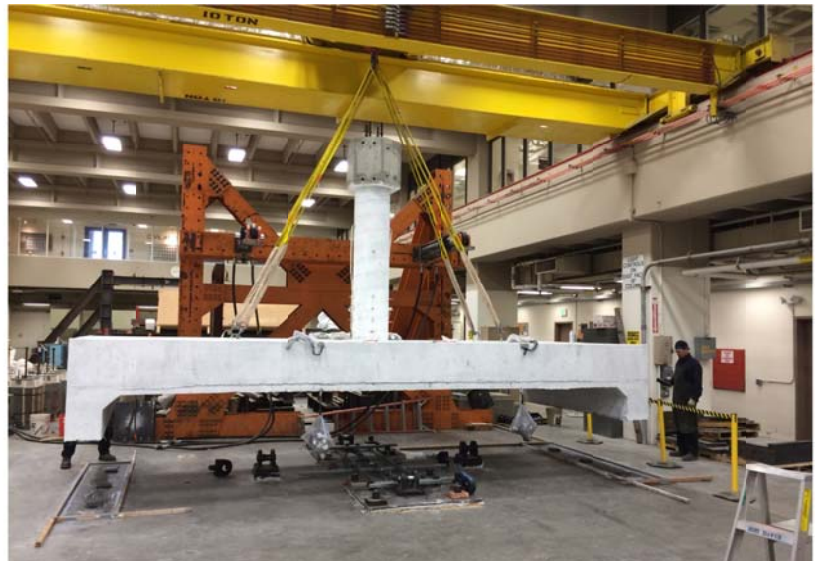
Figure D.4 Moving the first specimen from where it was constructed to where it was tested using the laboratory overhead 10-ton crane
