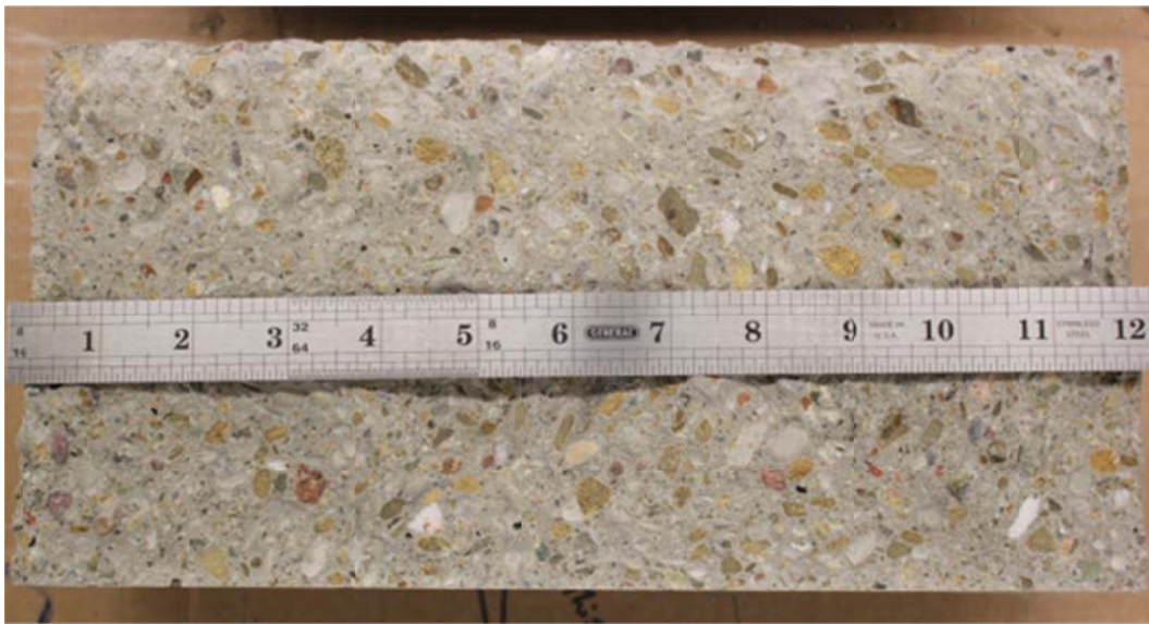
Figure 3.30 Close-up view of the concrete texture and aggregate size and distribution from a tested cylinder in splitting tension
