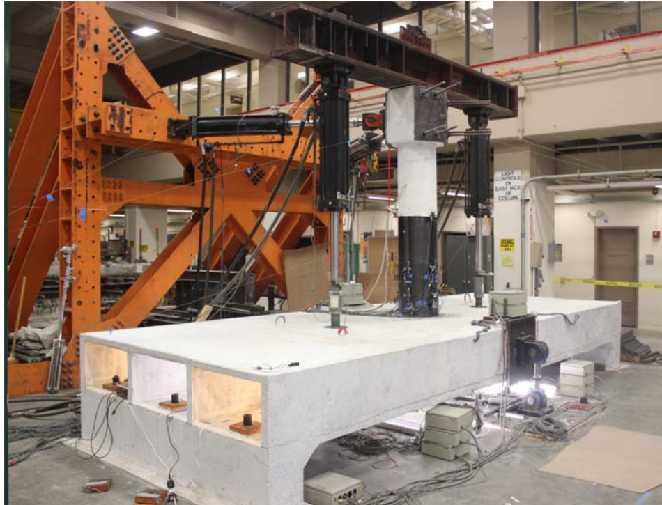
Figure 7.32 Test setup used for conducting HS trial tests for the repaired SP1
