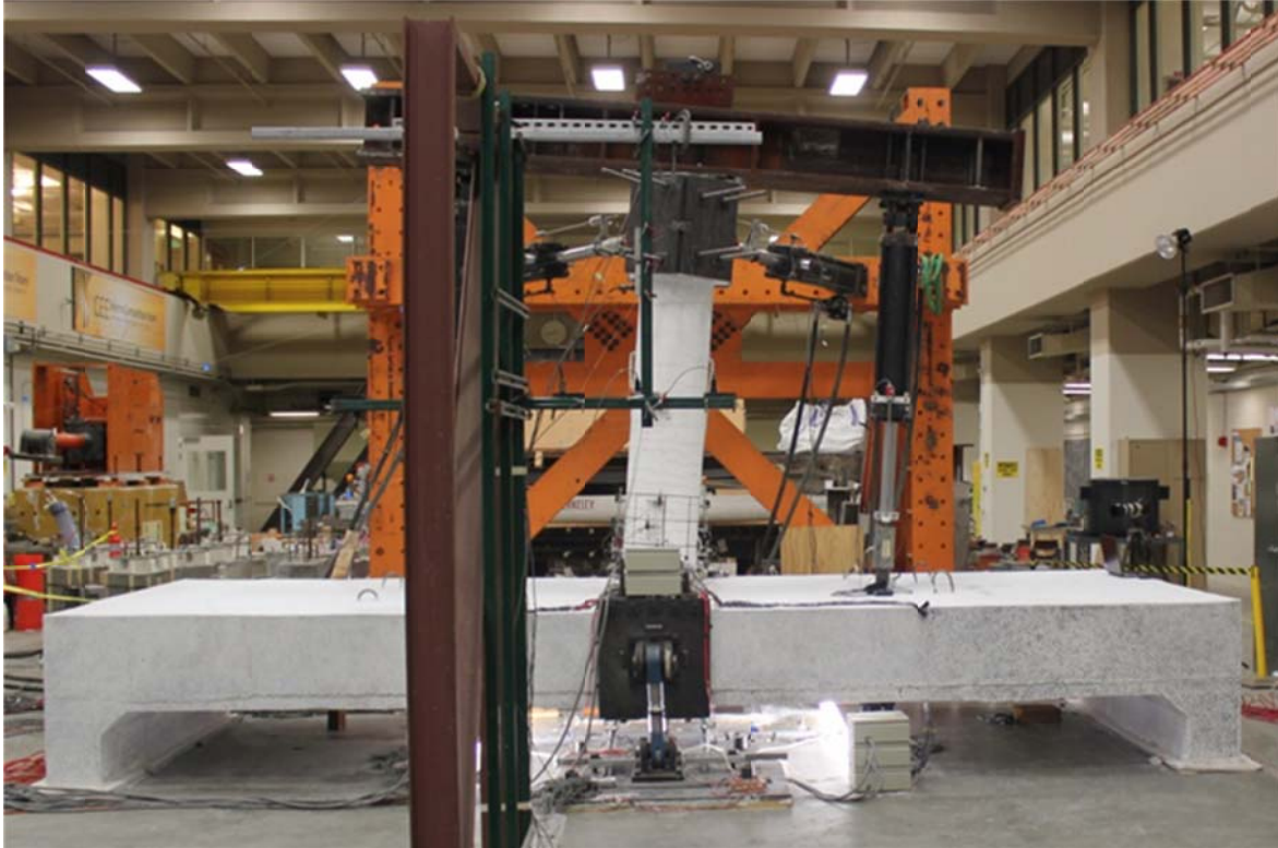
Figure 3.16 A view of first specimen test in progress under longitudinal cyclic loading
