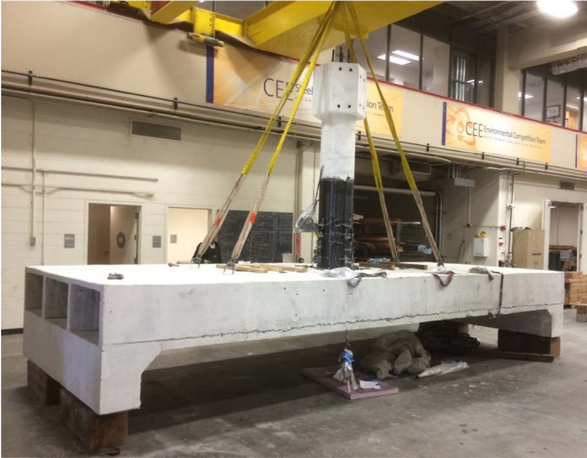
Figure 7.4 Physical experimental substructure (retrofitted SP2) used in the HS tests
