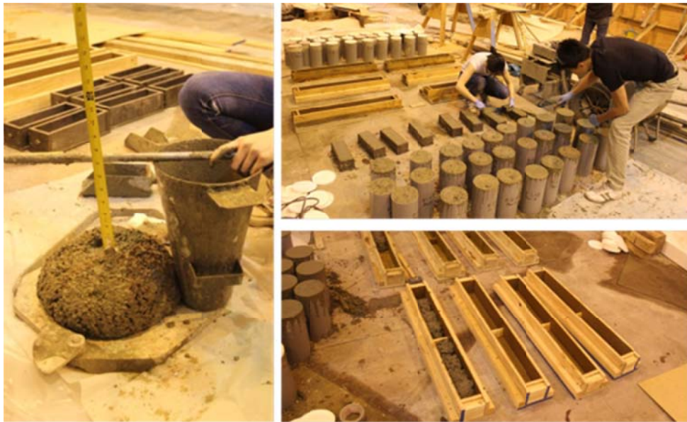
Figure 3.23 Slump test (left) and concrete sampling for material tests (top and bottom right)
