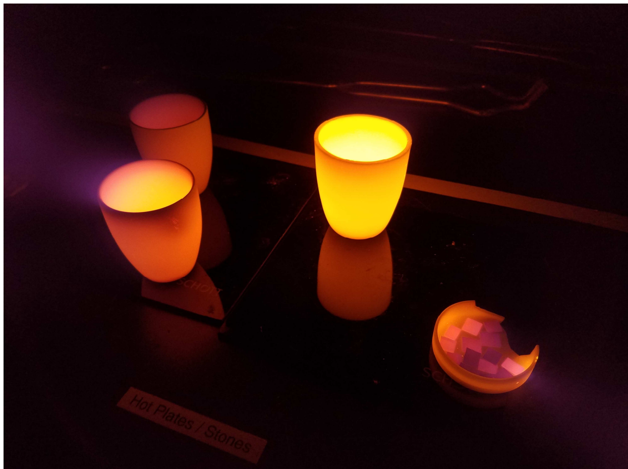
Figure 30 Post sintered alumina crucibles and dish.
