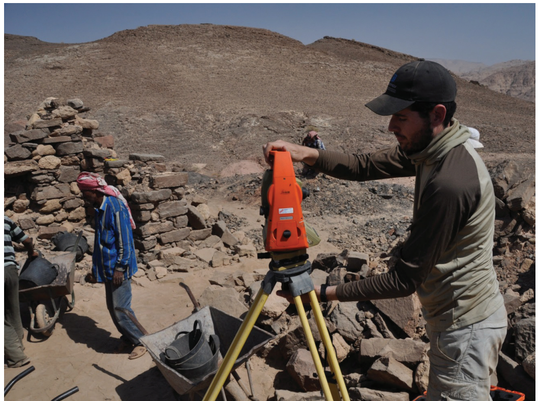
Figure 1. Example of total station deployed in the field for ArchField in Jordan's Faynan district. Photograph by T. E. Levy.
